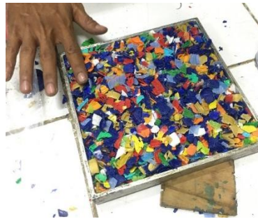
Figure 2 Process of Material Input into the Mold
