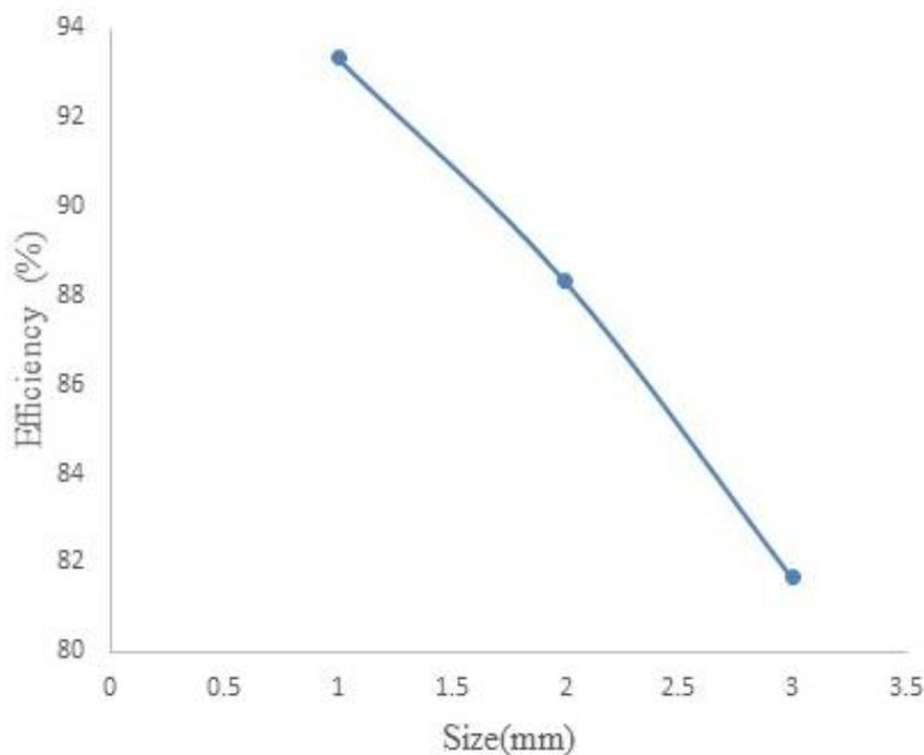
**Figure 2:** Relationship between slicing efficiency and tomato size
