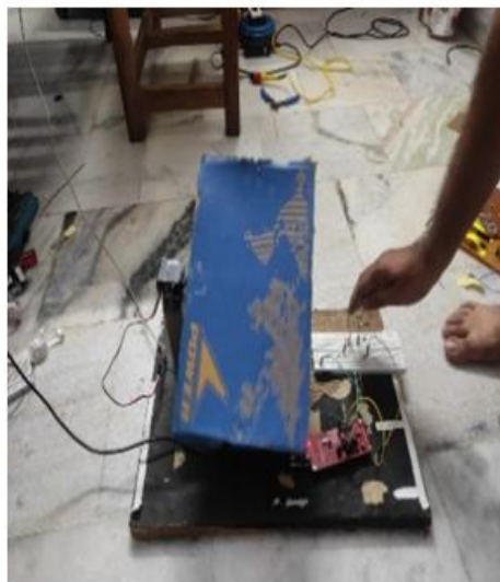
Fig.4.5. When Light intensity is maximum it stops moving
