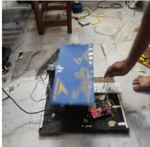
Fig. 4.4. When Light intensity is high on down side it starts moving
