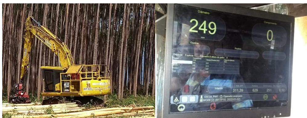
Figure 1. Forest harvesting machine and data acquisition system
