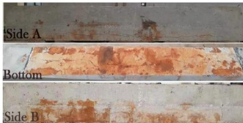
**Fig. 3.** Corrosion-induced cracks in beam PCB4
