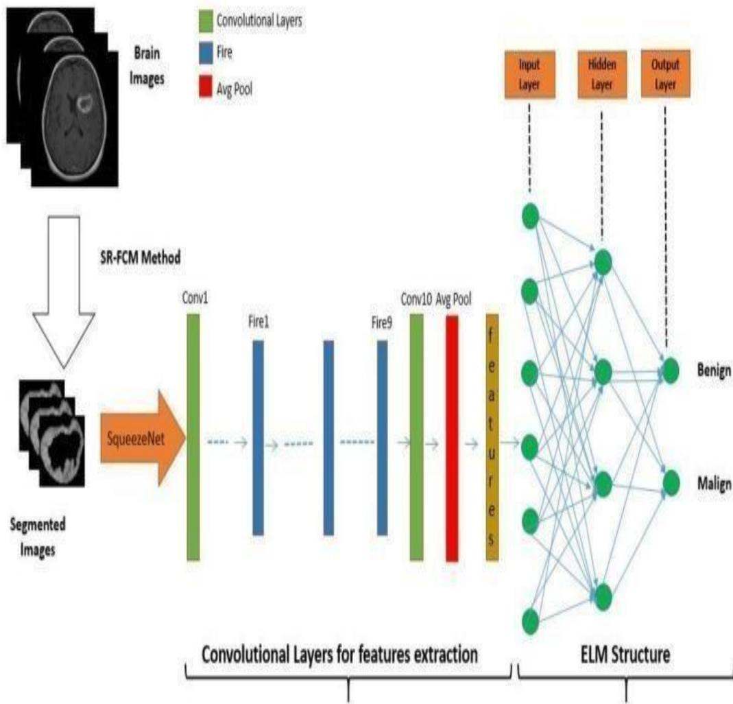
Fig 1.CNN Block diagram for tumor detection
