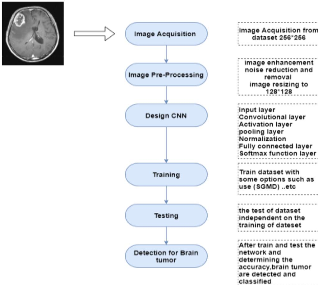
Fig 2. General Structure design for Brain Tumor Detection and classification
