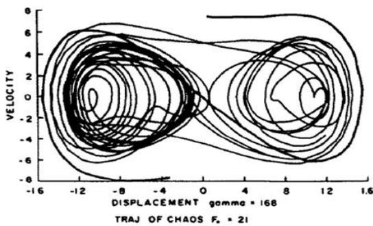
Figure 3: Phase plot trajectories [3].
