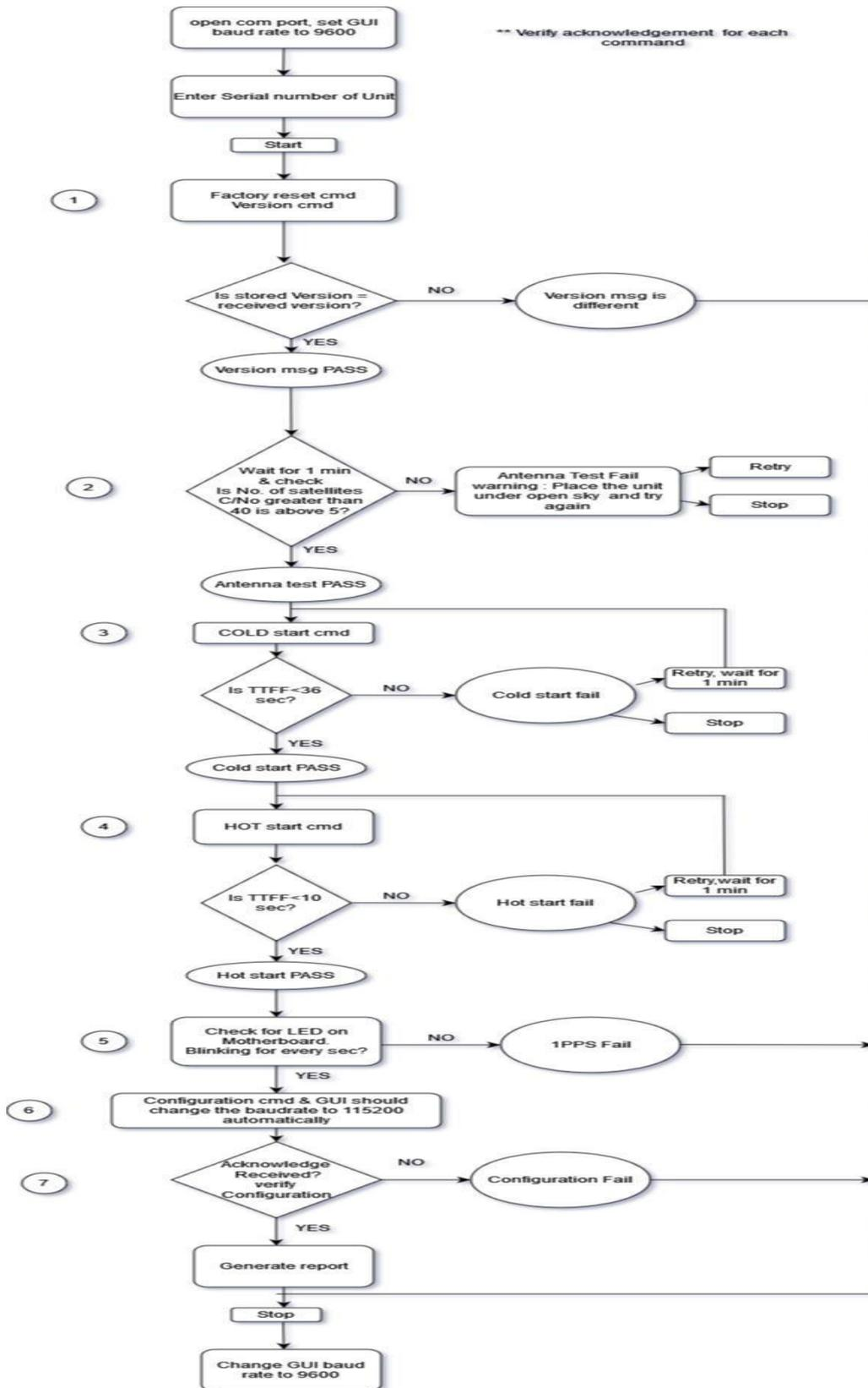
FIGURE 2. Flowchart of the steps to be followed to test the Smart Antenna device
