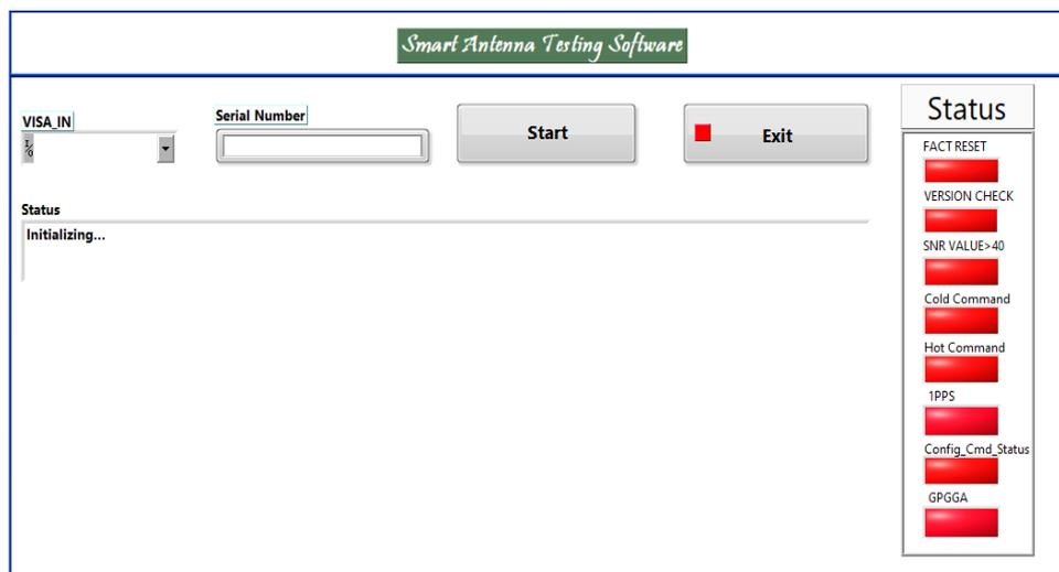
**FIGURE 3.** GUI developed to test the Smart Antenna device
