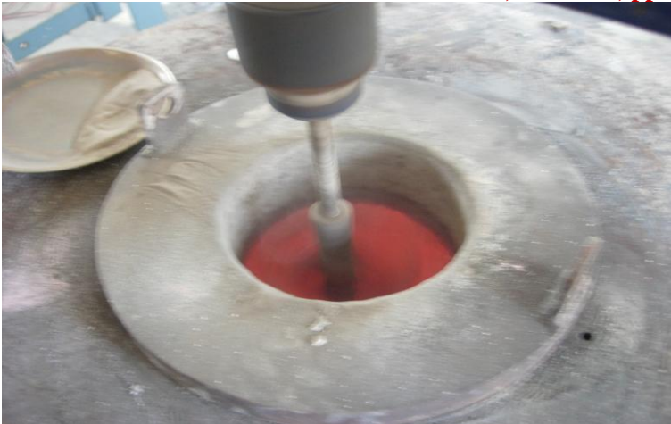
Figure1: A close-up view of the stir-casting process [21,22]
