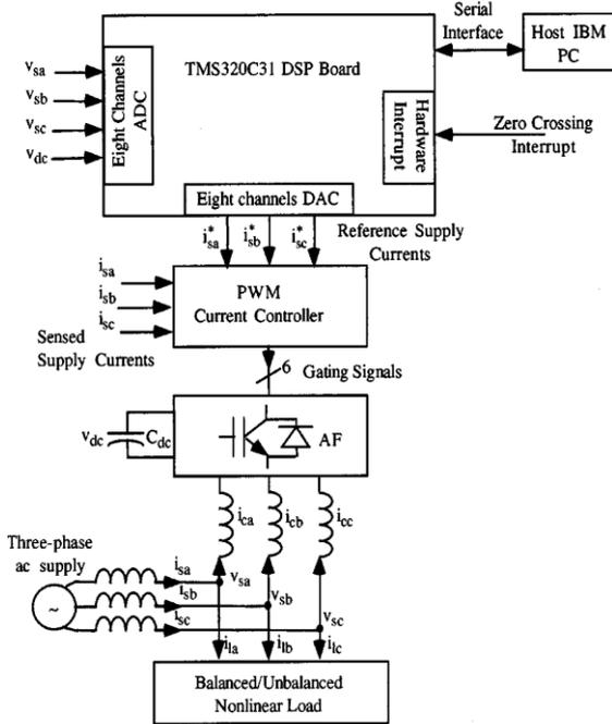
Figure 5. Digital signal processing (DSP) system hardware of the hybrid active filter.
