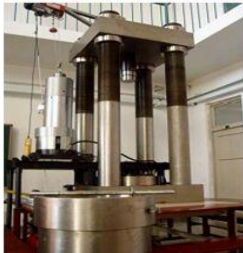
Fig.3 TAW-2000 microcomputer control electro hydraulic servo rock three axis testing machine system
