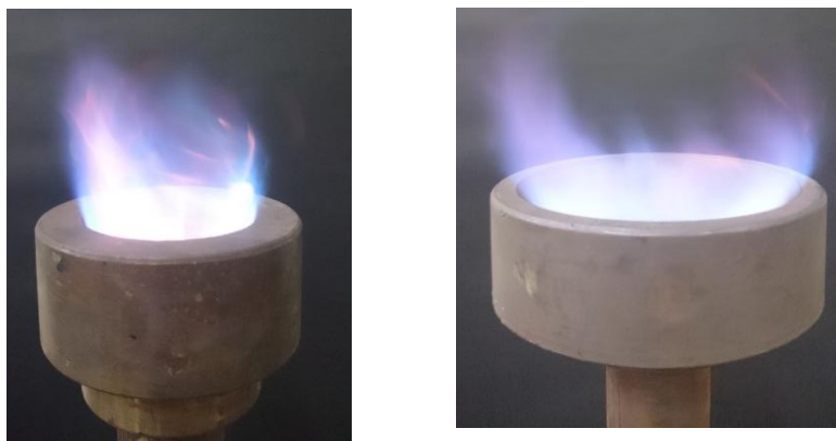
Fig. (12). TCP-IDF with 15^\circ diffuser at A/F ratio = 27, 45^\circ diffuser at A/F ratio = 27 Re inner air = 8069 and Re inner air = 8069, Re outer air = 8045, Re outer air = 8045.
