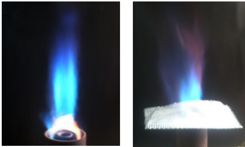
Fig. (17). Non- Swirling TCP-IDF Fig. (18). TCP-IDF with 1mm porous screen At A/Fratio= 27 and Re inner air = 8069 At A/Fratio= 27 and Re inner air =8069 Re outer air = 8045, Re outer air = 8045.
