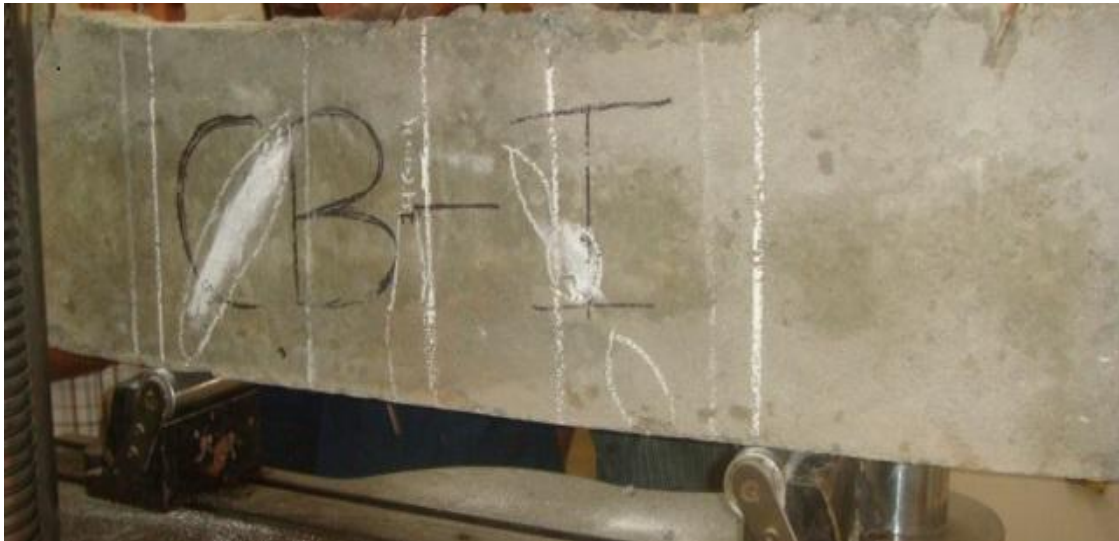
Fig 3.1 showing reinforced concrete beam before testing.
