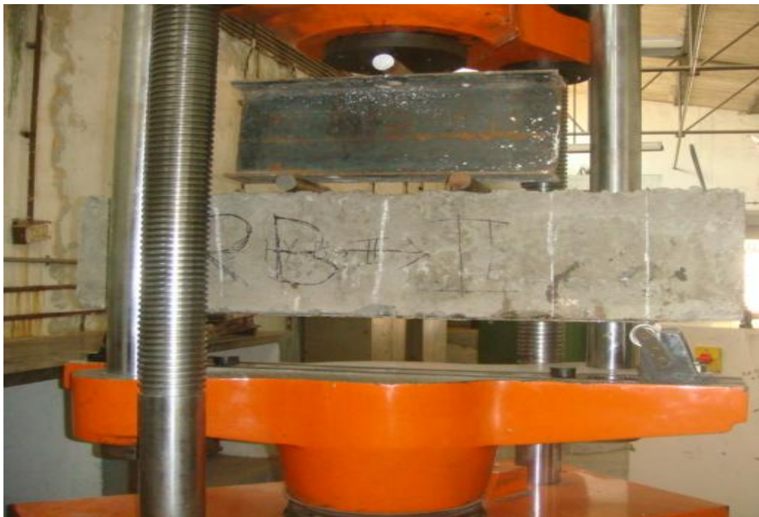
Fig 3.2 showing retrofitted reinforced concrete beam before testing.
