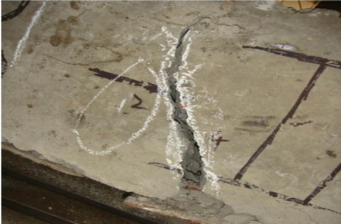
Fig 3.3 showing retrofitted reinforced concrete beam after testing.
