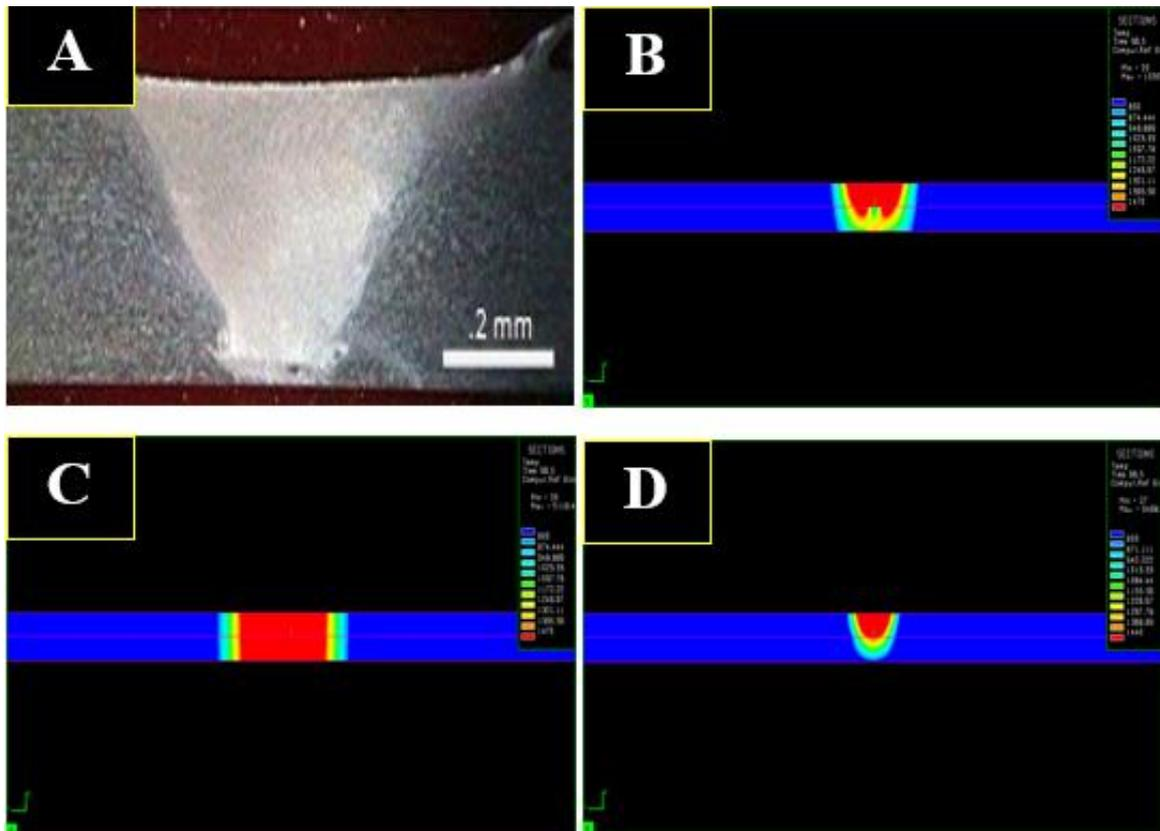
**Figure (3):** Comparison of cross-sectional area of x70 alloys weldment with simulated samples a) cross-sectional sample of weldment b) contour temperature of two-dimensional Gaussian cross-section c) three-dimensional Gaussian D) model of Goldak
