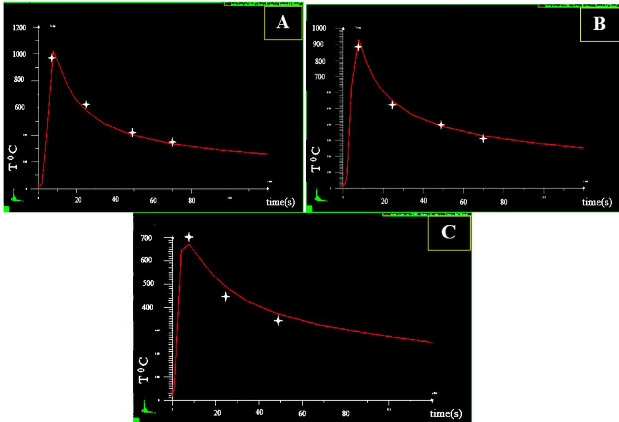
**Figure (6):** Comparison of experimental and simulated goldack model, solid line represents simulated data and the points representing the experimental data. A) Thermocouple 1 B) Thermocouple 2 and C) thermocouple 3
