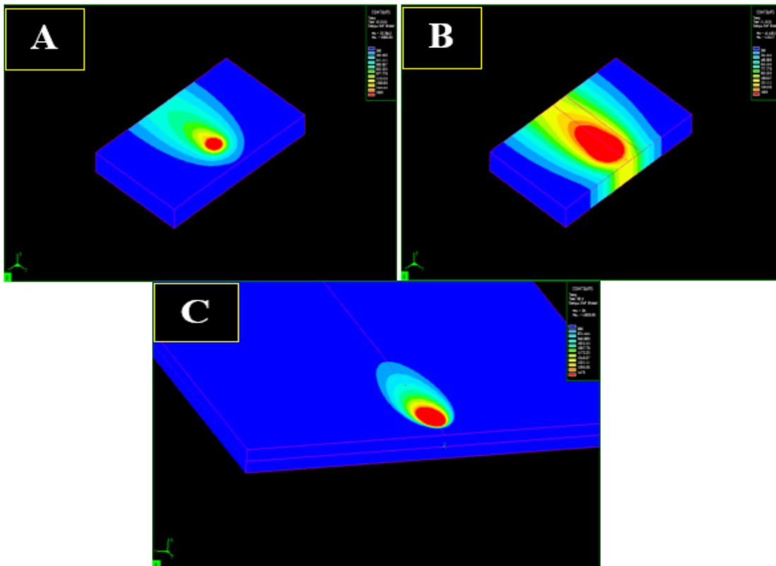
Figure (2): Contour of temperature distribution during the welding process a) two-dimensional Gaussian model, 10 seconds b) three-dimensional Gaussian, time of 11.33 seconds c) Goldak model, time: 96.5 seconds.
