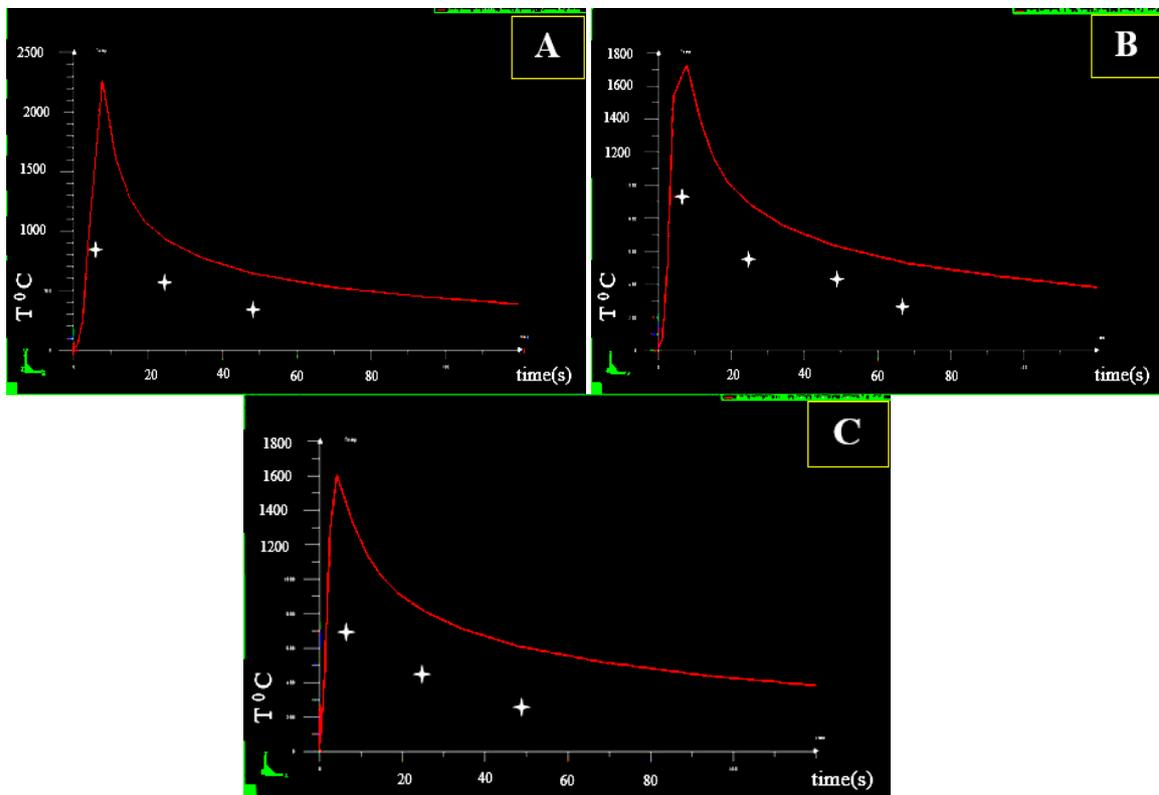
**Figure (5):** Comparison of experimental and simulated 3D- Gaussian model, solid line represents simulated data and the points representing the experimental data. a) Thermocouple 1 b) Thermocouple 2 and c) thermocouple 3
