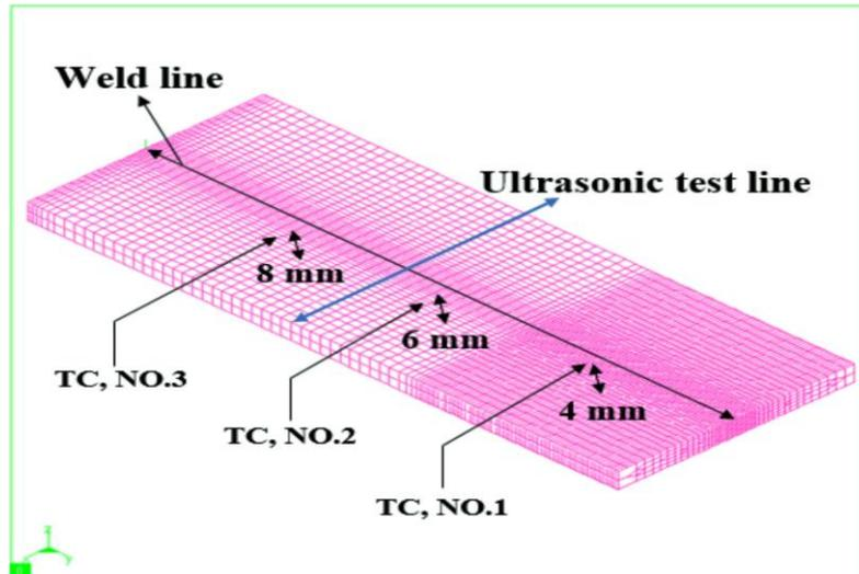
Figure (1): Schematic location of thermocouples (TC) in the path of welding and trajectory of conducting ultrasonic testing.
