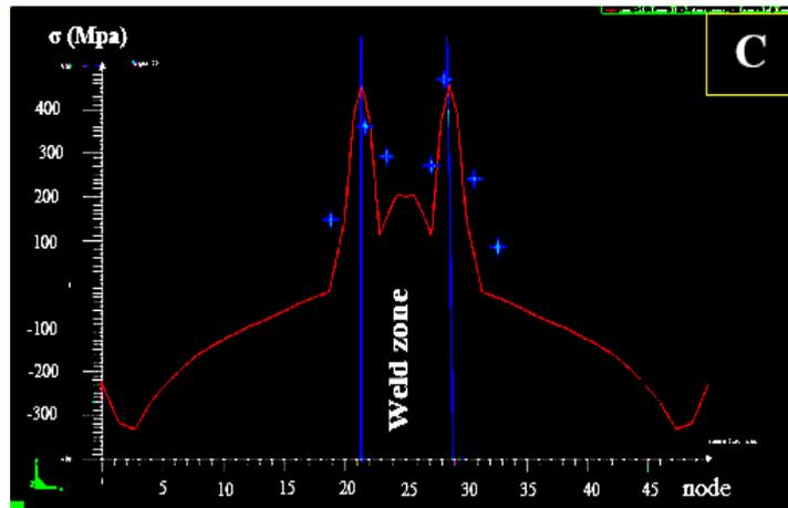
**Figure (7):** Comparison of data from residual stresses by software and ultrasonic testing, solid lines and simulated data and points represent simulated data and experimental data respectively. A) Residual stress in 2D-Gaussian B) 3D- Gaussian C) Goldak mode.
