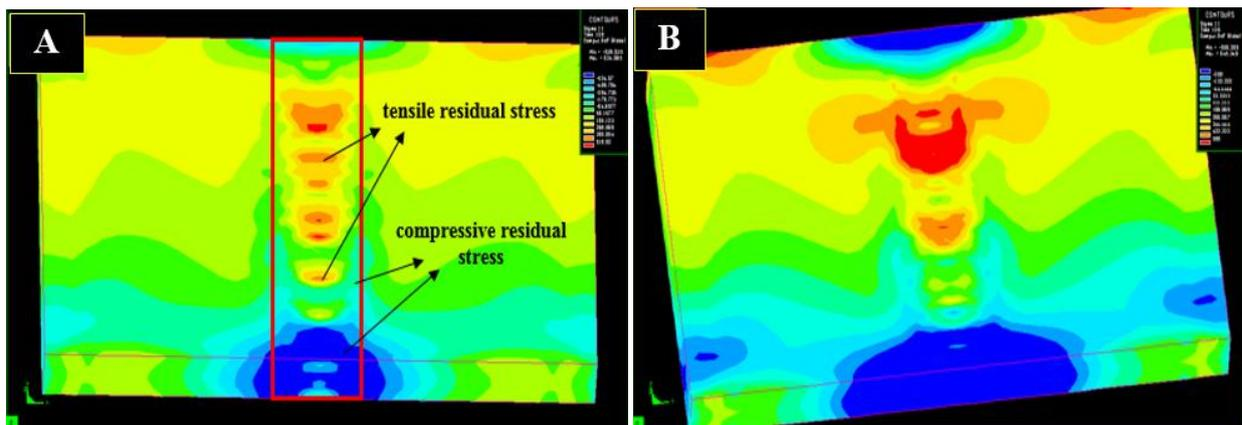
**Figure (8):** residual stress macrograph A) 2D- Gaussian model B) Goldak model
