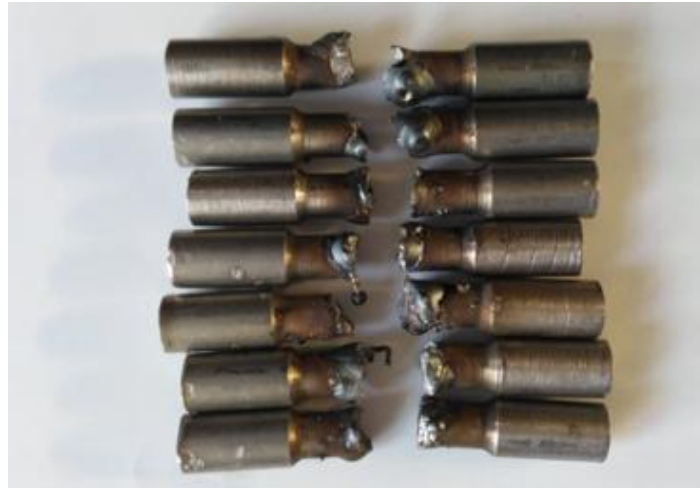
Fig 1: TIG welding Specimens after Fatigue Testing
