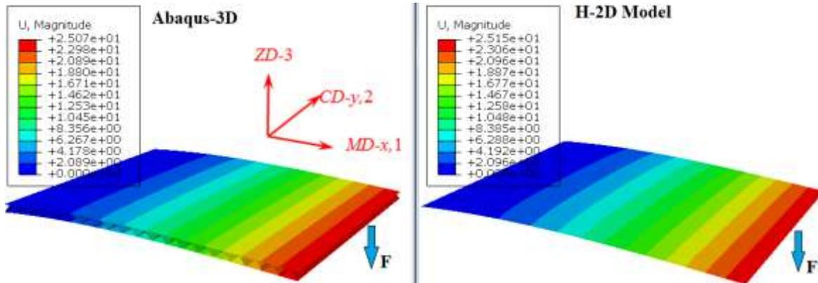
**Fig.6** Simulation of Abaqus-3D and H-2D Model in shear force on MD section
