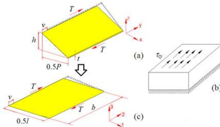
Fig. 3. The equivalent model to determine shear stiffness on CD section
