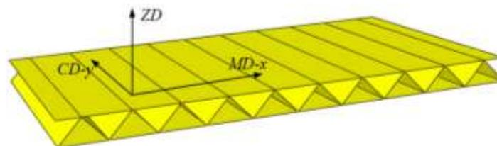
Fig. 1. The model of sandwich plate with folded core
