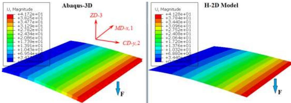
**Fig. 7** Simulation of Abaqus-3D and H-2D Model in shear force on CD section
