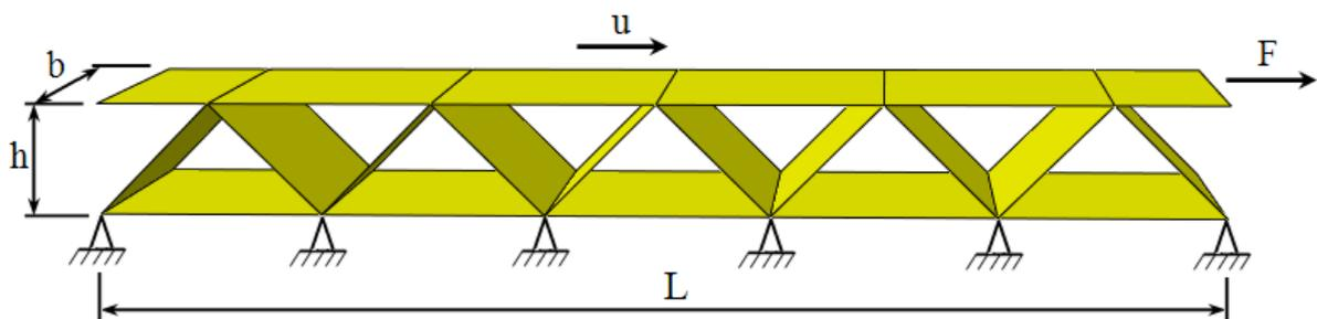
Fig. 4. The equivalent model to determine shear stiffness on MD section
