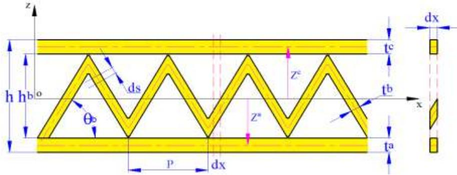
Fig. 2. Geometry of folded core plates
