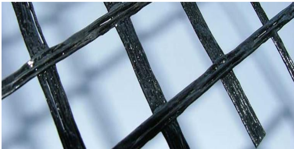
Fig. 3: Bonded Rod/Strap Geogrids
