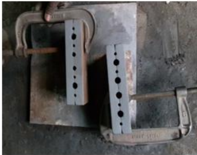
Figure 2: Cast iron die used to prepare the samples
