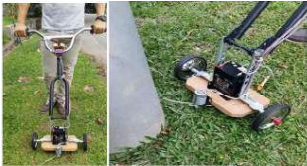
Figure 1. Battery operated simple lawn mower(RubentheranSivagurunathan et al. 2017)
