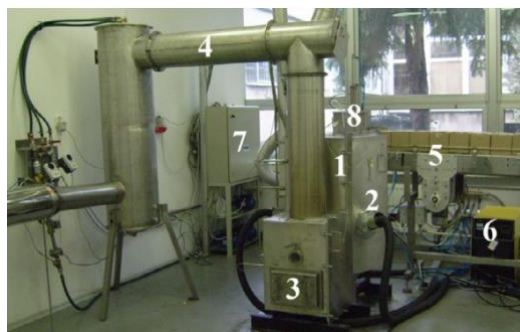
Fig. 6 Thermal arc plasma reactor (1) plasma reactor, (2) plasma torch, (3) molten product collector), (4) fume exhaust chimney, (5) waste conveyor, (6) plasma energy source, (7) PLC automation and data collection apparatus cabinet and (8) waste feeder.
