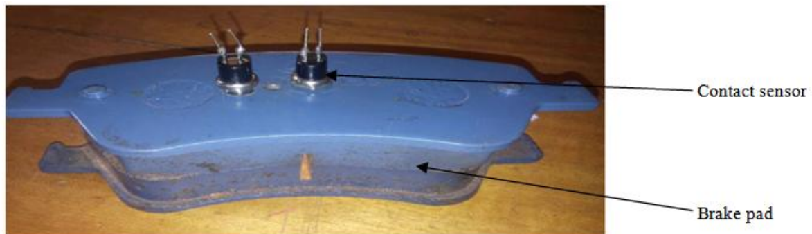
Fig.5: Brake pad with the contact sensor
