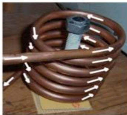
Fig 4. Principle of Induction Heating
