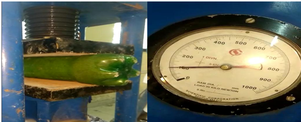
Figure 3 . Compression Test On 2 litre Bottle (Specimen 3) with Result (Specimen 3)
