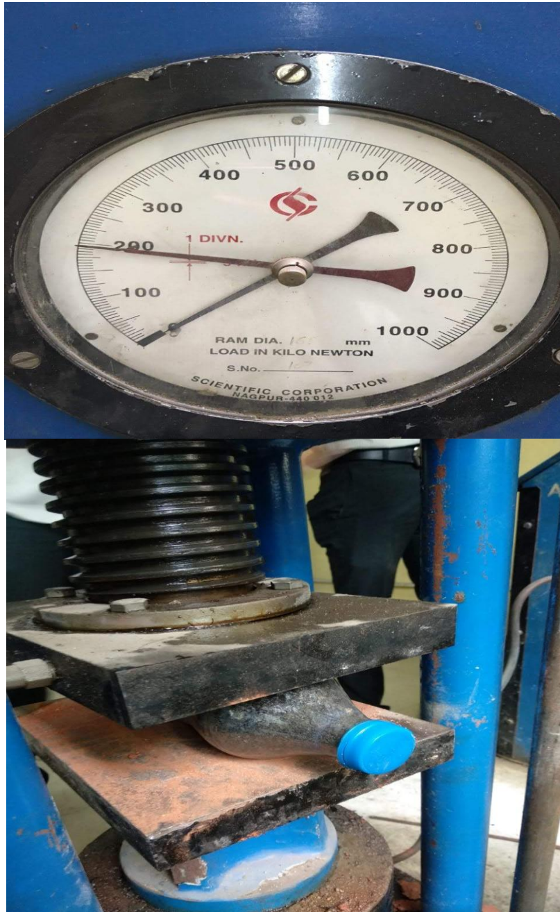
Figure 4 . Compression Test On 1 litre Bottle M-sand(Specimen 4) with Result (Specimen 4)
