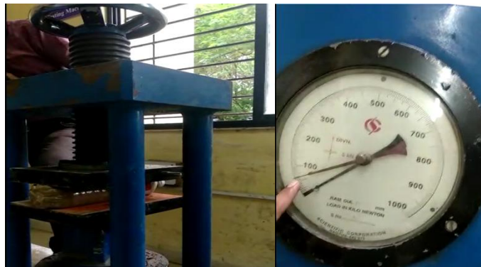
Figure 2 . Compression Test On 1litre (Specimen 2) with Result (Specimen 2)
